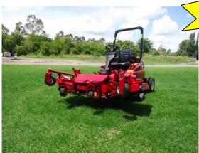
The Shibaura CM364 with 84 inch Flex Deck is an excellent professional outfront mower with a 35hp Shibaura 3-cylinder Diesel Engine
